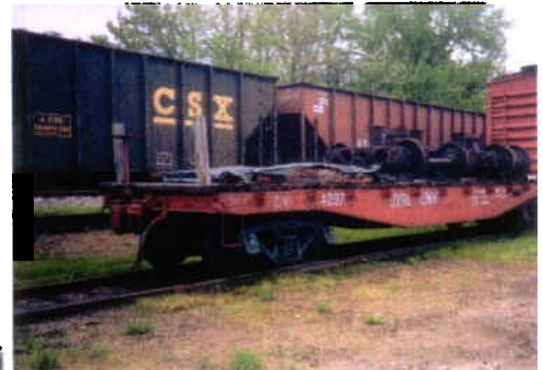
Central Vermont CV 4287, 40'6" fish belly flat car is on the CT East RR Museum track with CV boxcar 43022. The hopper cars are on a siding of the New England Central (former Central Vermont) mainline in Willimantic CT. The right hand hopper is NYC 490163 and has the Conrail logo -- go figure!!
